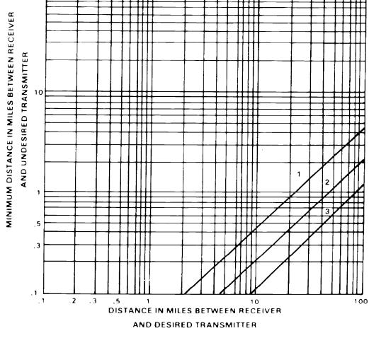
Figure B-11. Interference chart for AN/VRC-12 low power versus SINCGARS (adjacent channel, 50 kHz spacing).
