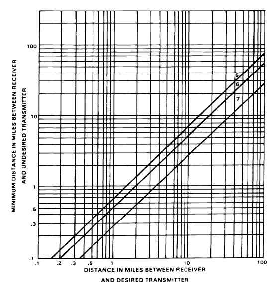
Figure B-3. Interference chart for SINCGARS versus SINCGARS (cochannel). (continued)
