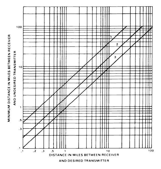
Figure B-8. Interference chart for AN/VRC-12 high power versus SINCGARS (cochannel).
