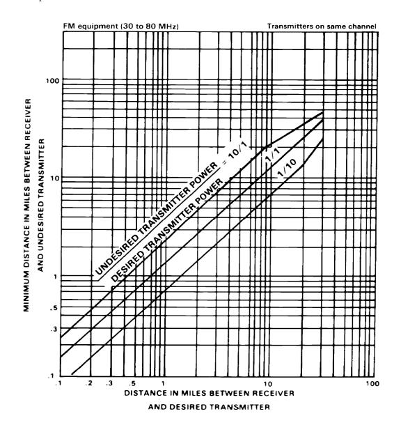
Figure B-1. Interference chart (FM same channel) for AN/VRC-12 series radios.
