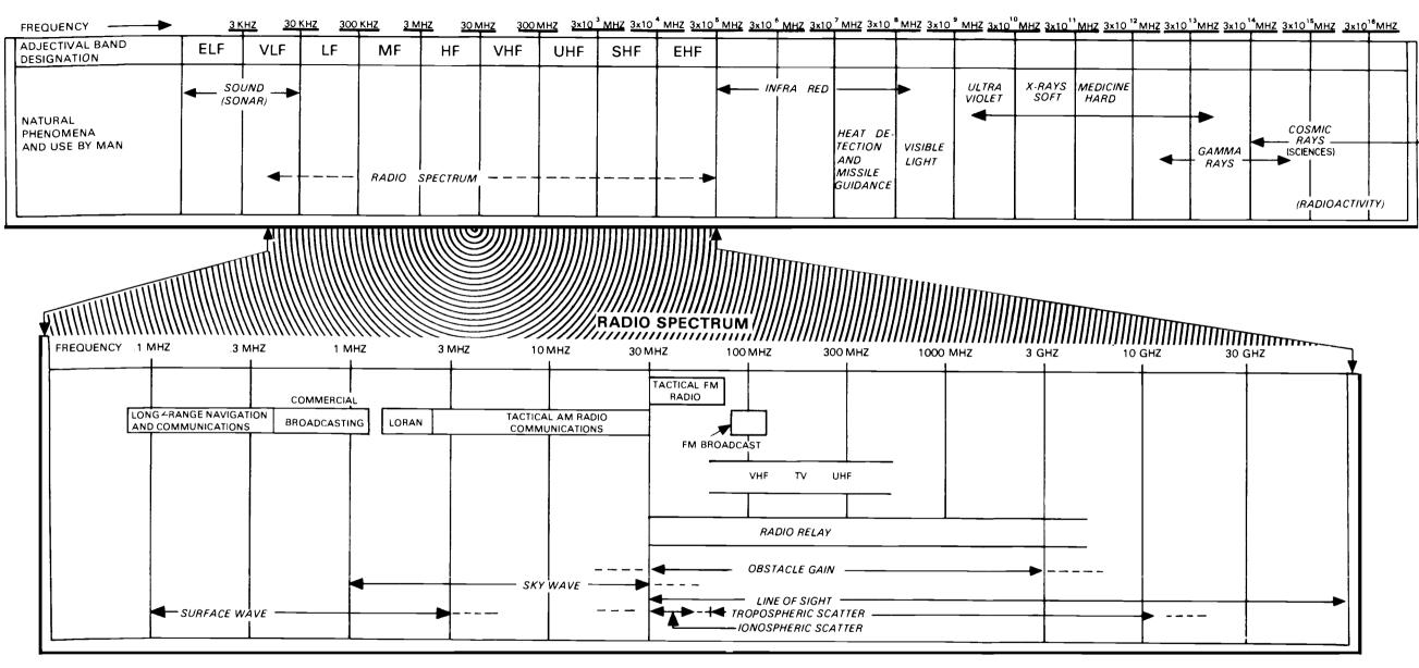
Figure 1-2. The electronmagnetic spectrum with the radio portion highlighted.
