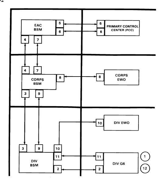
Figure A-12. UHF single-channel satellite coordination flow.
