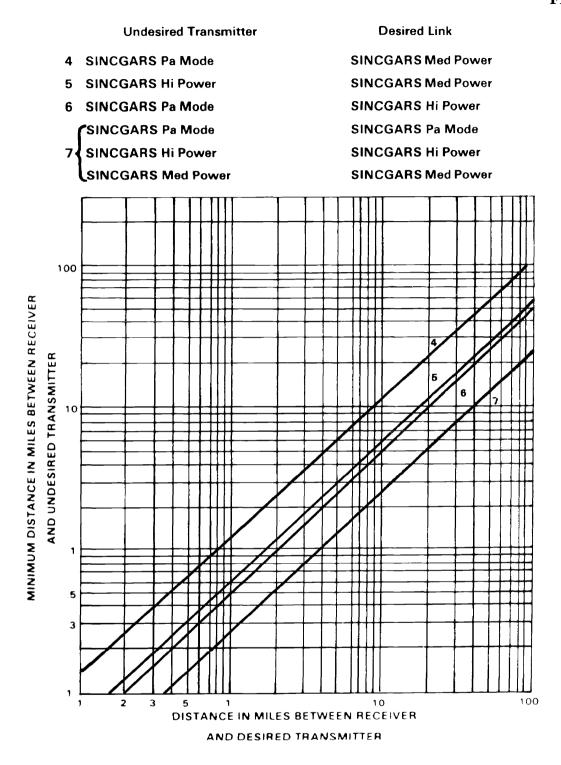
Figure B-4. Interference chart for SINCGARS versus SINCGARS (adjacent channel, 25 kHz spacing). (continued )
