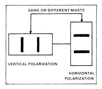
Figure G-1. Cross-polarization.
