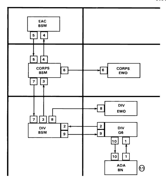
Figure A-15. VULCAN radar coordination flow.
