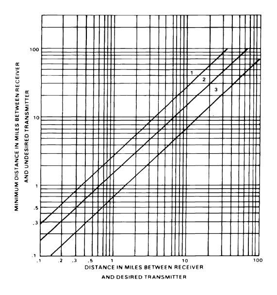
Figure B-5. Interference chart for SINCGARS versus AN/VRC-12 low power (cochannel).
